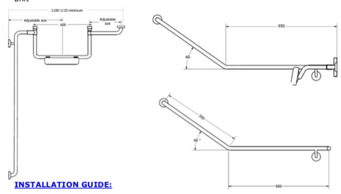
These units are to be surface mounted and are subject to compliance to Building Code of Australia and/or AS 1428.1 for height location and fitment for disabled/accessible use as may be applicable, which is the responsibility of the installation contractor.
